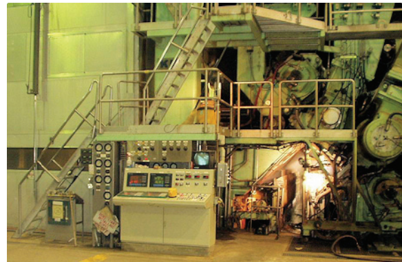
Figure 3. The press section at the mill included obsolete and malfunctioning 1970's era controls.
